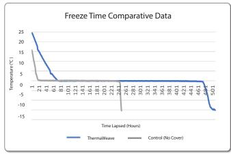
\* Pallets are placed in a container freezer set to -25°C. Test ended when product reached -15°C
