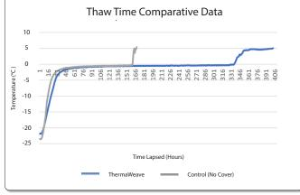
\* Frozen 500lt Pallecon filled with water with Pallet Covers on them, removed from freezer and placed in warehouse.
