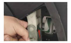
8. After releasing the chain link, make sure that the sliding window is fully closed. The safety switch of the control unit will unlock only after the sliding window is fully closed. (When the sliding window is opened, the yellow light flashes and prompts "please close the sliding window" on the central control screen. When the sliding window is closed, the green light flashes.
