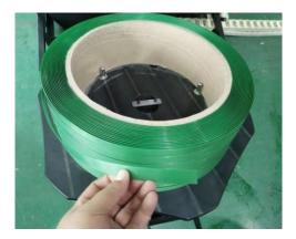
4. Fold up the disc arm with the strap roll again in its vertical position as shown in the picture .
