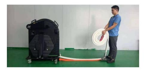
1. Push the new chain in the opposite direction ( note the number of new chain , the correct number is 210 ) . When pushing about two meters , it is clearly felt that the chain is occluded with the main machine gear , and then start up and adjust the equipment to " changing chain mode " . Then press the joystick in the forward or backward direction until the chain is fully retracted into the machine
