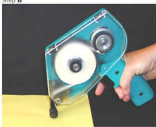
Release trigger and continue to pull dispenser away to break 'adhesive tissue' at desired length, do not lift dispenser whilst pulling away.
