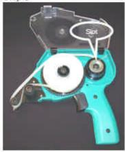
Thread the 'white liner paper' into the slot in the 'take up spool'.
