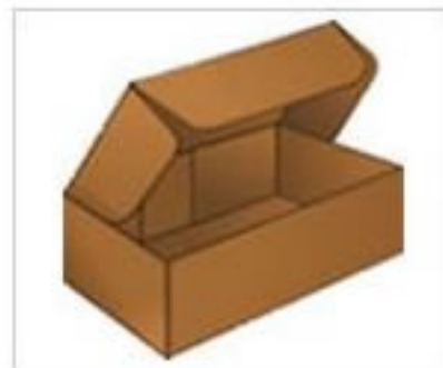
FOE full depth tuck in top, with cover flaps
