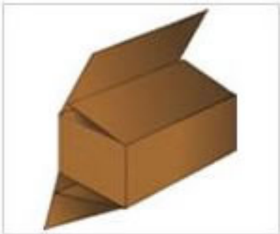
FFSC - Full flap slotted container
