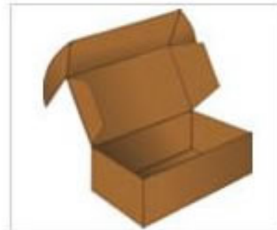
Fold over end, with cover flaps and ears
